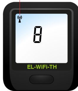
4) RECEIVED SIGNAL STRENGTH INDICATOR (RSSI) (VALUE BETWEEN 0 & 10)
